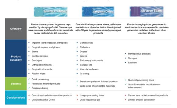
See "Industry Overview—Sterilization overview" for more detail about these technologies. We provide gamma irradiation services at 23 of our facilities, EO processing services at 17 of our facilities and E-beam irradiation services at eight of our facilities.
